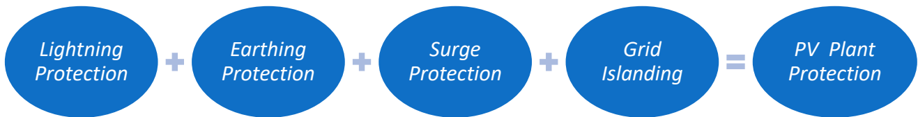
Figure 35: Protections in a PV plant
